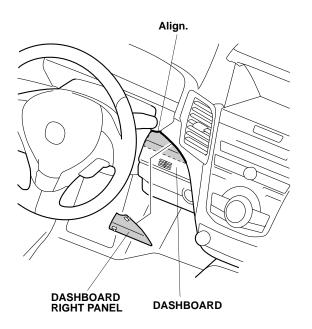
12. While applying light pressure against the dashboard right panel, carefully remove the adhesive backings.
