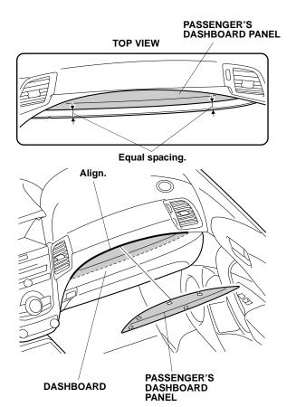
26. While applying light pressure against the passenger's dashboard panel, carefully remove the adhesive backings.
