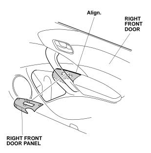
22. While applying light pressure against the right front door panel, carefully remove the adhesive backings as shown.
