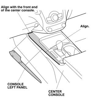
16. While applying light pressure against the console left panel, carefully remove the adhesive backings.
