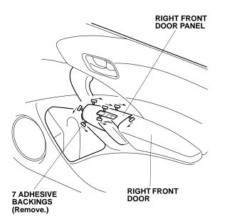
23. Using your hand, firmly press the right front door panel against the right front door.
