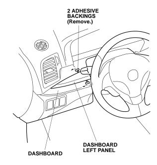
9. Using your hand, firmly press the dashboard left panel against the dashboard.
