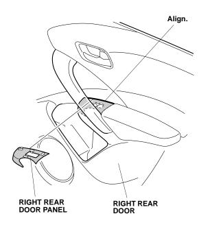
31. While applying light pressure against the right rear door panel, carefully remove the adhesive backings.
